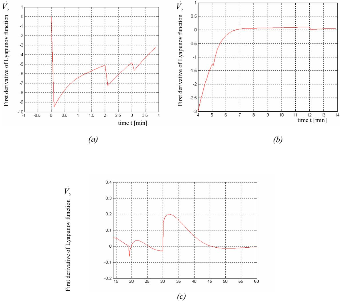
Fig. 4. First derivative  $\dot{V}_2$  of Lyapunov function (30) at  $t \in [0, 4]$  is shown in (a). (b) illustrating the behavior of  $\dot{V}_2$  for  $t \in [4, 14]$  and subfigure (c) illustrating the behavior of  $\dot{V}_2$  for  $t \in [19, 60]$ , respectively.
