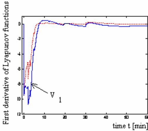
Fig. 2. Current first derivatives  $\dot{V}_1$  (blue) and  $\dot{V}_2$  (red) of Lyapunov functions (30) and (33) at  $t \in [0, 60]$ .
