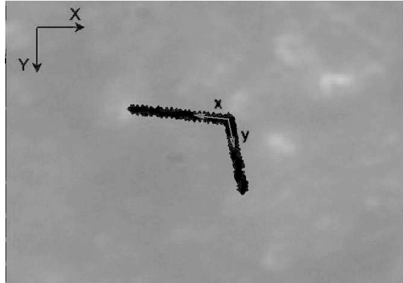
Fig. 7. Picture of the accumulated displacements of the end-effector during the voltage change
