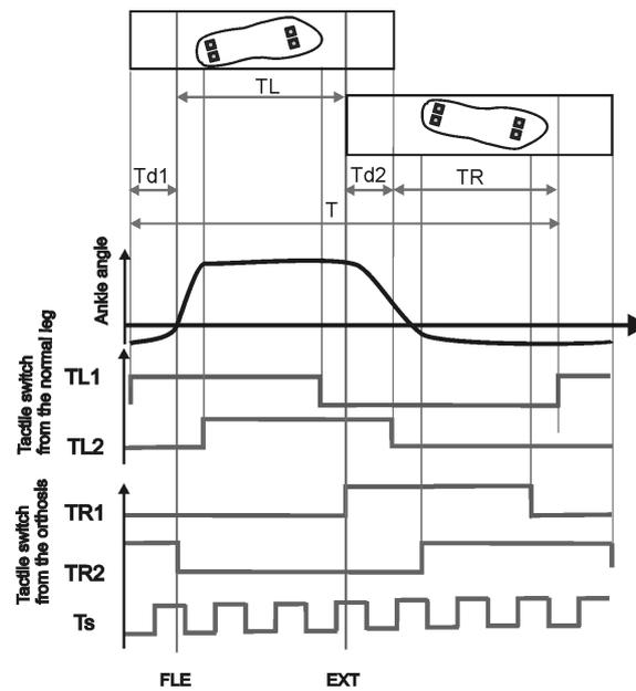
Fig. 4. Signals from the external sensors
