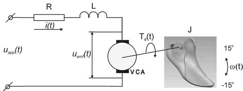
Fig. 7. A simple model of a DC actuator driving an inertial load
