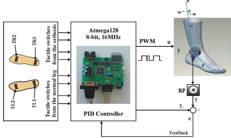
Fig. 5. Autonomous Control System with Active Ankle-Foot Orthoses
