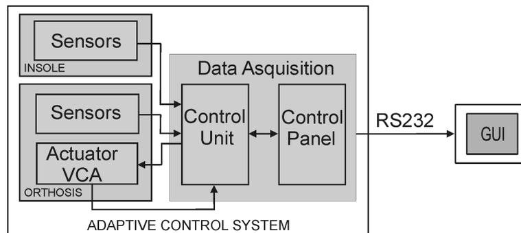
Fig. 1. Autonomous control and monitoring system with active ankle-foot orthoses
