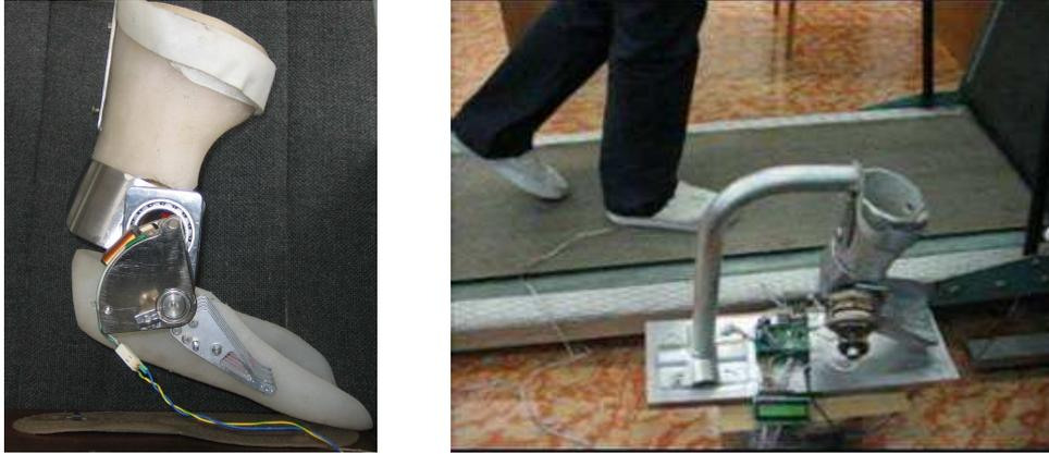
Fig. 8. AAFO with the hinge joint and attached laterally direct drive actuator
