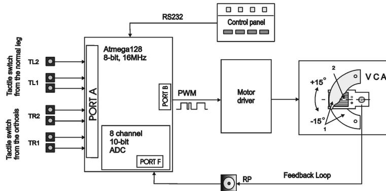
Fig. 3. ATmega128 controlling a VCA
