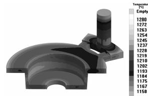
Fig. 14. Temperature field during the solidification
