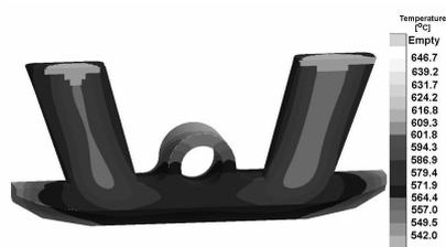
Fig. 5. Temperature field during the crystallization
