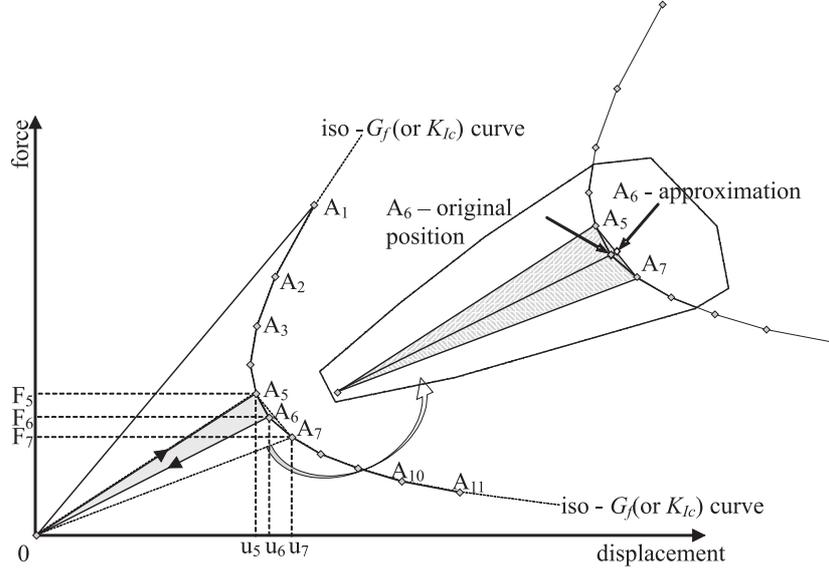
Fig. 2. Typical force-displacement curve obtained by LEFM principles
