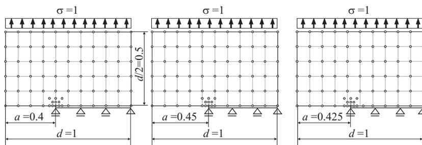
Fig. 5. EFG numerical models for different crack lengths
