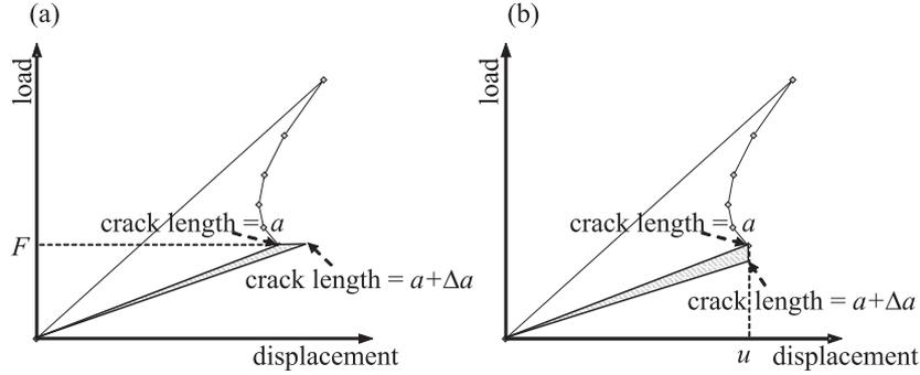
Fig. 3. Virtual incremental fracture process: (a) At constant load; (b) At constant displacement
