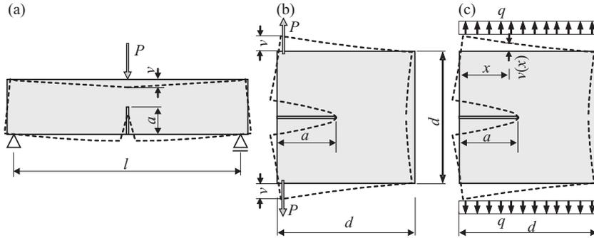
Fig. 1. Plane structures of thickness  $b$  with a pre-existing crack of length  $a$
