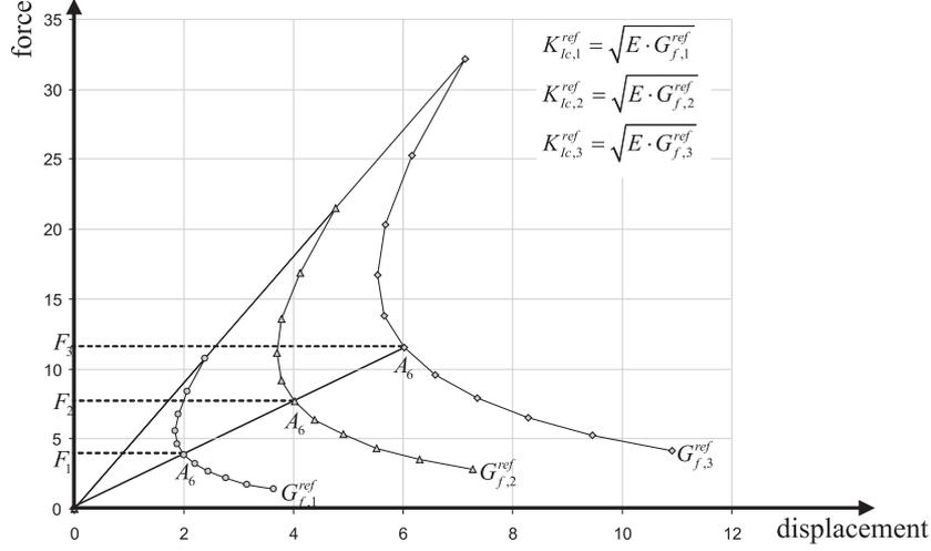
Fig. 4. Typical load-displacement curves obtained by LEFM for different values of fracture energy
